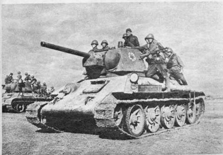
New turret to hold T-34's long-barreled 76.2-mm. gun has bulging "cheeks" on either side of gun mantlet. T-34 has a long sloping bow and broad tracks. Five double bogie wheels are large and dish-shaped.
